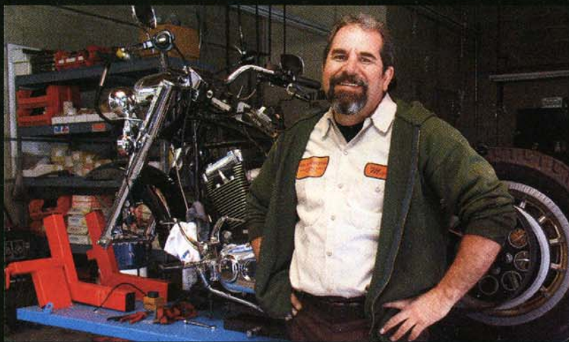
Mark chopped his single-post car hoist up into a bike lift. It almost sits flush to the shop's floor.
