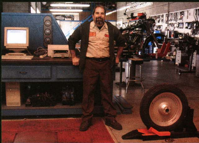
Mark chopped his single-post car hoist up into a bike lift. It almost sits flush to the shop's floor.
